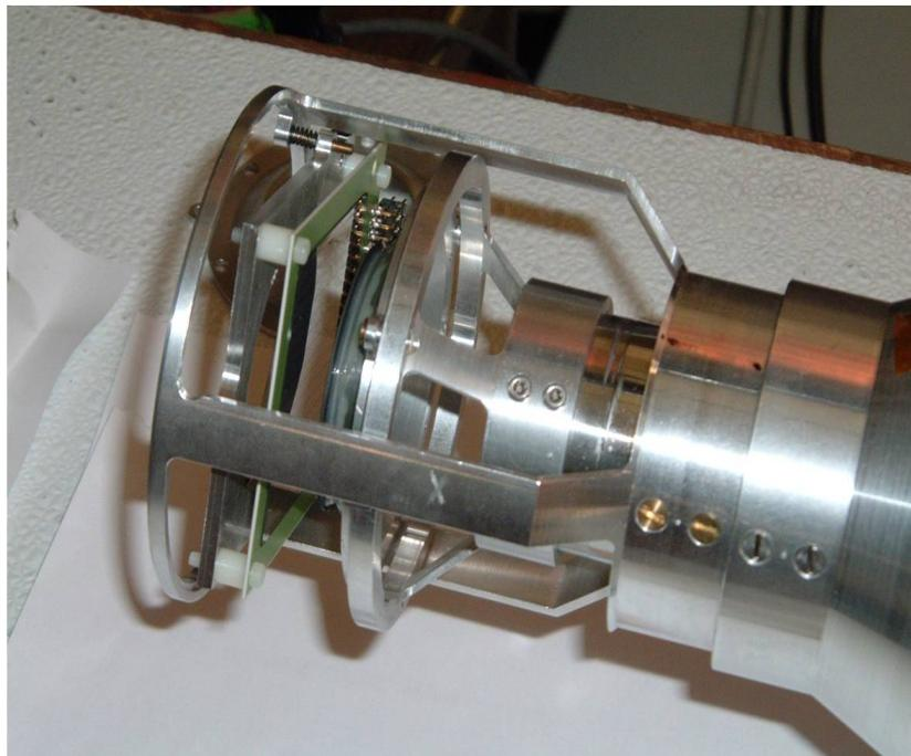
**Plunger with a  $500\mu\text{m}$  carbon target and a double sided,  $16\times 16$  strip,  $300\mu\text{m}$  silicon detector on a ceramic mount from Micron Semiconductor.**
